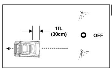
Release intermittent trigger switches or turn off continuous setting on solution switch approximately 1 foot before ending cleaning pass.
